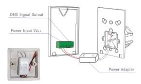
5 Embed the upper touch panel into the baseplate and then tap the button to press into the slots.
