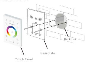
1. Install the back box into the wall. Typical boxes as below:
