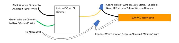
NOTE: Must use appropriate components that comply with local codes if installed outdoors (weather-proof connectors, cord covers, enclosures, etc). This product is NOT field-cuttable, which would void the IP rating and warranty.
