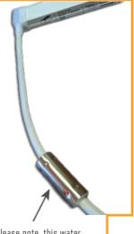
Please note, this water wicking barrel is on each lead wire, and helps prevent water from running down the wire into the fixture. Length is 1.25", diameter is .5". Do not remove it.
