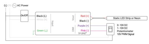
• The on/off switch is on the input side. 0-10V/1-10V controls dimming only, not on/off function
